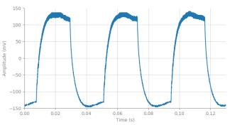
Figure 4 Typical measurement for a 23 Hz square modulation signal in medium sensitivity mode
