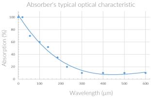
Figure 1 Absorption vs frequency of black coating
