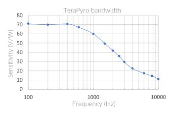
Figure 7 Sensitivity as a function of the gate frequency
