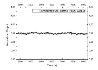
Figure 3 Stable regime for a 25% duty cycle sub-modulation corresponding to 1.1 mW output power on a 2.5 THz QCL
