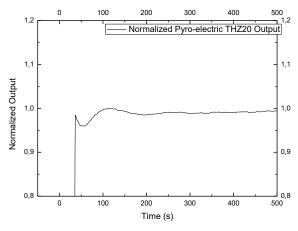
Figure 2 Stabilisation regime for a 50% duty cycle sub-modulation corresponding to 1.7 mW output power on a 2.5 THz QCL
