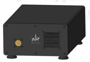
The NLIR MIR Spectrometer is based on a novel measurement scheme that upconverts the MIR light to near-visible light. Silicon-based near-visible light detectors are far superior to MIR light detectors in terms of detectivity, speed and noise. The NLIR upconversion technology therefore brings these attractive features, and the advantages that follow, to the MIR regime.
