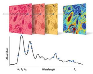
A high-resolution spectrum is collected simultaneously at every image pixel position (230,400 pixels per FOV) in less than 45 seconds.
