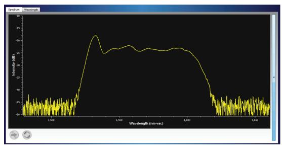
The Low resolution option is available to better measure the spectral features of broadband lasers. The spectrum of a broadband SLED using Low resolution is shown below. Even with a bandwidth of 100 nm, the noise floor is about 30 dB below the spectrum's peak intensity.
