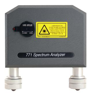
Since fiber is not readily available for infrared wavelengths, the laser under test enters the IR and MIR versions of the model 771 through a 2-3 mm input aperture. To facilitate alignment to the instrument, the internal HeNe reference laser is emitted from the input aperture as a visible tracer beam. The laser under test is simply superimposed on the tracer beam to optimize alignment. This is accomplished by using the three adjustable-height legs ( $\pm$  0.25") of the 771 system.
