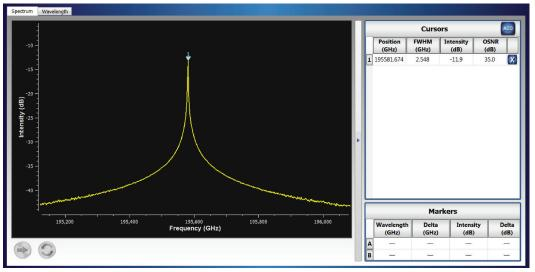
These two spectra are of the same narrow band laser. The first spectrum is generated using Standard resolution. The measured bandwidth is 4.233 GHz and the optical signal-to-noise ratio (OSNR) is greater than 40 dB at 1 nm away from the peak. The High resolution algorithm is used for the second spectrum. Higher spectral resolution is achieved as evidenced by the measured bandwidth of 2.548 GHz. However, the noise floor drops gradually near the peak thereby reducing the OSNR measurement.
