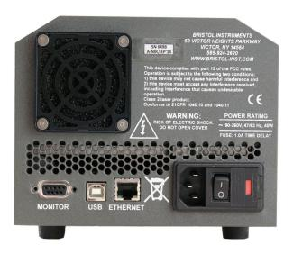
The spectral information generated by the 771 Laser Spectrum Analyzer is transferred to a PC directly using a USB interface or via a local area network using Ethernet. Analysis is done with the system's Windows-based software, or relative intensity versus wavelength data can be collected and saved to a file using a \*.csv format for analysis with other graphing programs. Data can also be transferred using a convenient library of commands for custom or LabVIEW programming.
