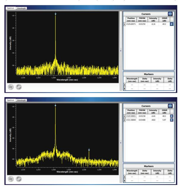
The ORR of the 771 Laser Spectrum Analyzer is also dependent on the intensity of the laser under test. The ORR rises as the input power increases from the minimum detectable power, and then levels off as the electronic noise floor begins to rise with the input signal.
