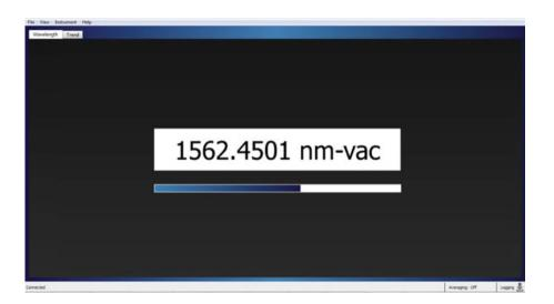
Wavelength data can also be logged to a file using a \*.csv format for analysis with other graphing programs. Data can be logged by number of measurements, amount of time, or continuously until the logging is stopped manually.
