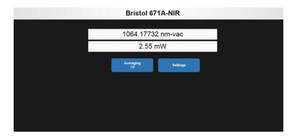
The display application offers customizable features similar to the 671 system software. Measurement units can be expressed in wavelength (nm or  $\mu$ m), wavenumber (cm<sup>-1</sup>), or frequency (GHz or THz). Power for the VIS and NIR versions is reported in a linear (mW) or logarithmic (dBm) format. The displayed wavelength and power values can be updated with each new measurement, or a rolling average of as many as 100 measurements can be calculated automatically.
