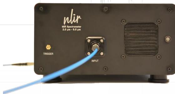
The NLIR S2050 MIR Spectrometer is based on a novel measurement scheme that upconverts the MIR light to near-visible light. Silicon-based near-visible light detectors are far superior to MIR light detectors in terms of detectivity, speed and noise. The NLIR upconversion technology therefore brings these attractive features, and the advantages that follow, to the MIR regime.
