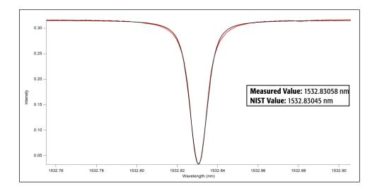
Wavelength data (red) measured with the model 871A-NIR as a laser tunes through an absorption of acetylene gas (NIST SRM 2517a). A Voigt curve fit of this data (black) gives a measured absorption wavelength of 1532.83058 nm. The published NIST value of 1532.83045 nm is well within the wavelength meter's accuracy of ± 0.3 pm.
