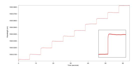
Laser wavelength vs. time of a tunable external cavity diode laser. With its speed, the 871 system has the capability of measuring the laser's tuning characteristics (wavelength overshoots then settles to target, as shown in inset detail of single step).
