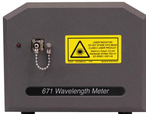
Since fiber is not readily available for infrared wavelengths, the laser under test enters the IR and MIR versions of the model 671 through a 2-3 mm input aperture. To facilitate alignment to the instrument, the internal HeNe reference laser is emitted from the input aperture as a visible tracer beam. The laser under test is simply superimposed on the tracer beam to optimize alignment. This is accomplished by using the three adjustable-height legs ( $\pm 0.25''$ ) of the 671 system.
